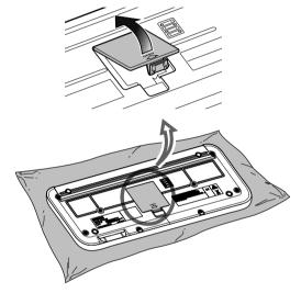
3 Insert the four new batteries, being careful to follow the polarity markings on the inside of the compartment.
