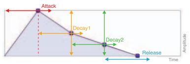
*Release* represents the amount of time from *Decay2* (and normally indicates how long it takes after the key is released until the sound fades away completely); however, if the amplitude for *Decay2* is set to "0", it represents the duration from *Decay1*.
